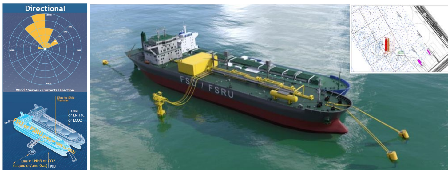
Figure 10 : Fixed heading jetty-less system for DIRECTIONAL environment or PROTECTED site
