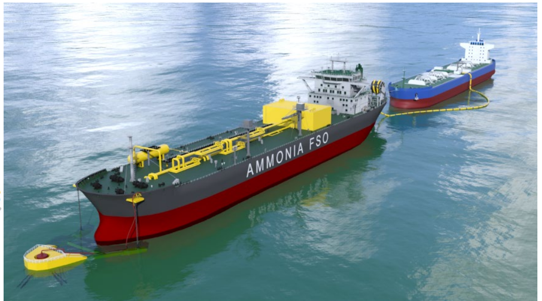
Figure 12 : weathervaning jetty-less system for OMNIDIRECTIONAL environment in open sea
