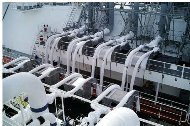
Figure 6: typical current use of ammonia hoses in quasi-static application
